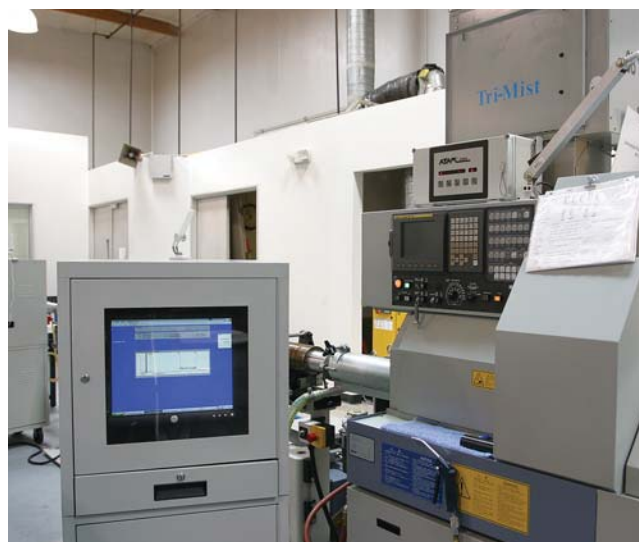
Atam throughput optimization system at work. The Atam, a black box sitting on top of the Star, monitors system vibration and yields reports as required.
