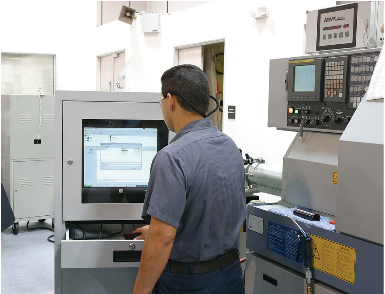
Jesus Guillen, setup machinist, uses Shop Floor Automation's Predator DNC software to download a program to one of Implant Direct's 26 Star turning centers.
