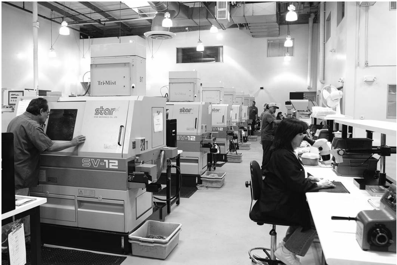
Line up of Star SV-12 turning centers at Implant Direct LLC. In the first two and a half years the company bought a new Walter CNC tool grinder, 14 new Star SV-12 turning centers and 12 new Star SB-16 turning centers. The machines are all equipped with live tooling, automatic bar feeders, on the floor PCs, Shop Floor Automation's Predator DNC software, TriMist filters and Atam throughput optimization systems.
